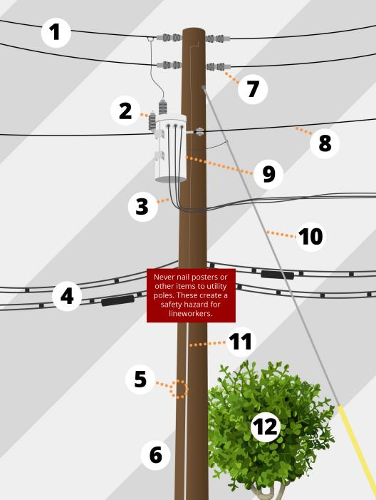
**Primary wires** run on top. Each carry at least 7,200/14,400 volts of electricity from a substation.
